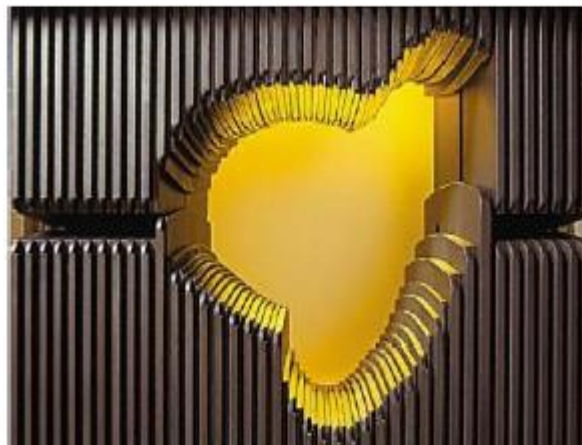
Figure II.25. Le collimateur mutilâmes MLC
