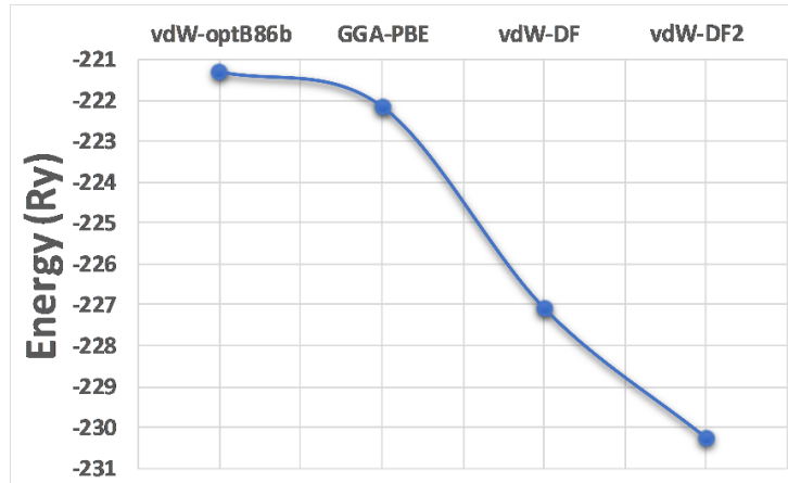
Figure III.4: Calculated total energy ( E_{\text{total}} ) for monolayer phosphorene as a function of different van der Waals corrections (vdW-optB86b, vdW-DF and vdW-DF2) as compared to the GGA-PBE approximation.
