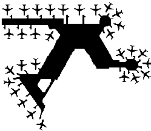
Figure 38 Example of gate disposition
