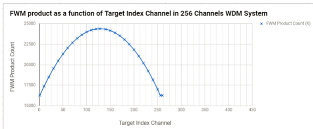
Fig. 7. FWM product as a function of Target Index Channel in 256 Channels WDM System
