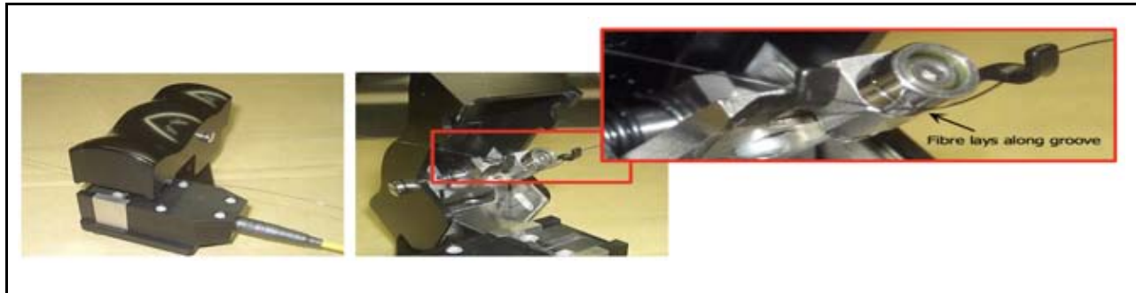
Figure A1.28 Close-up for an optical clip-on coupler. Adapted from [53]
