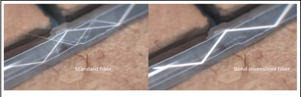
Figure A1.3 Microbending [20]
