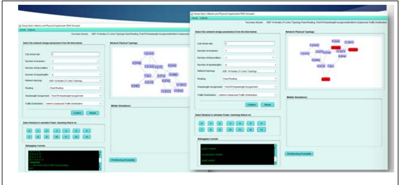
Figure 3.25 The developed simulator for dynamic RWA algorithm - NSFNET 14 Nodes 21 Links
