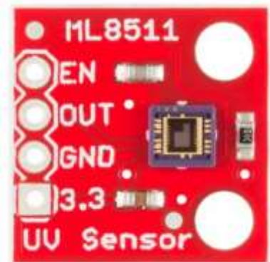
Figure 103: ultra-violet light sensor
