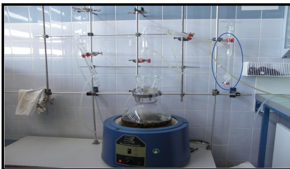
Figure 2: Montage d'hydrodistillation (Clevenger)
