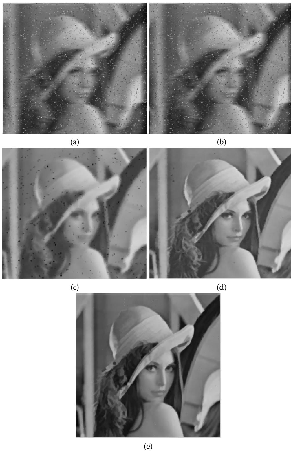
Figure 3.4: Comparison of "Lena" outcomes using the different methods : (a) original (b) degraded by blur and impulse noise \rho = 0.3 (c) MHNN (d) RMHNN (e) CHN.
