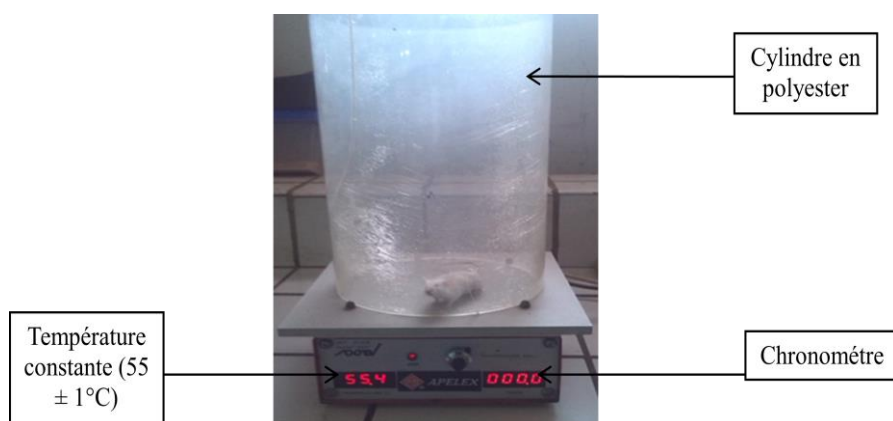
Figure 11: Dispositif de la plaque chauffante
