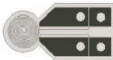
Figure 39: Probe used in the TPS method to thermally excite the sample and measure the temperature of the heating filament
