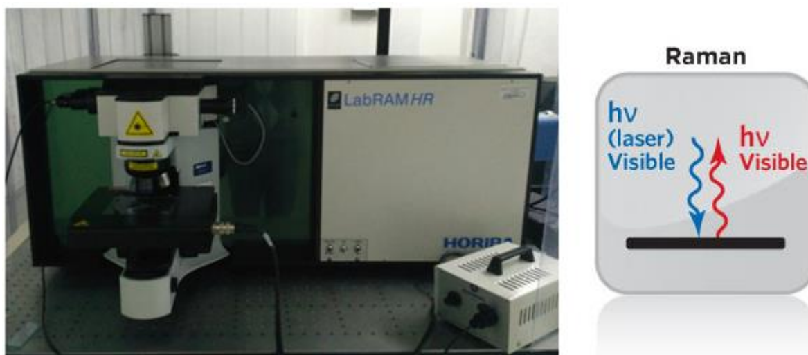
Figure 56. Raman spectrometer Horiba Jobin-Yvon LabRam HR800 from Horiba Company
