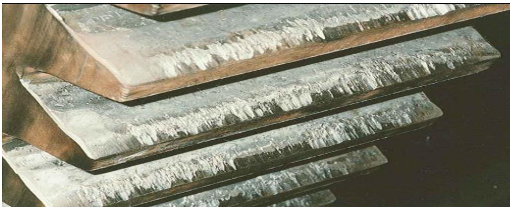
Figure 1.7 Grippage de dentures.
