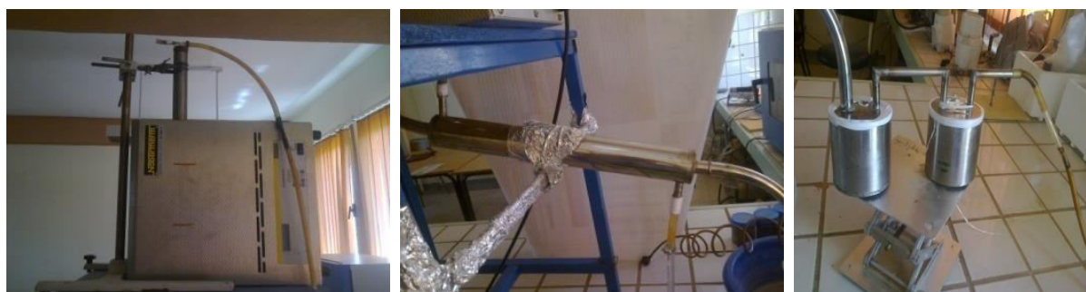
Figure II-5: Left: tubular reactor inserted in a furnace; Middle: condenser; Right: two collecting.
