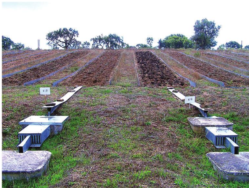
Picture 1: Soil erosion experimental plots under some crop rotations (Experimental Station in Polytechnic Institute of Castelo Branco/School of Agriculture) (Duarte, 2017)
