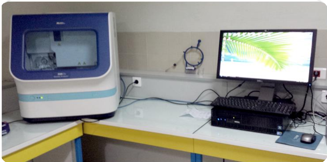
Figure 16: The automatic sequencer (Genetic Analyzer 3500 Dx) available in the Genetic laboratory ( CHU fez).
