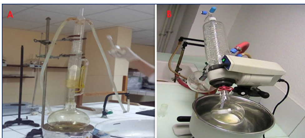
Figure 11 . A) Appariel Soxhlet.
