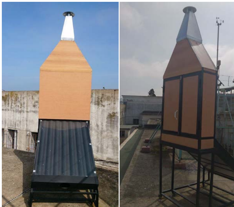
Figure III- 3: Séchoir solaire indirect
