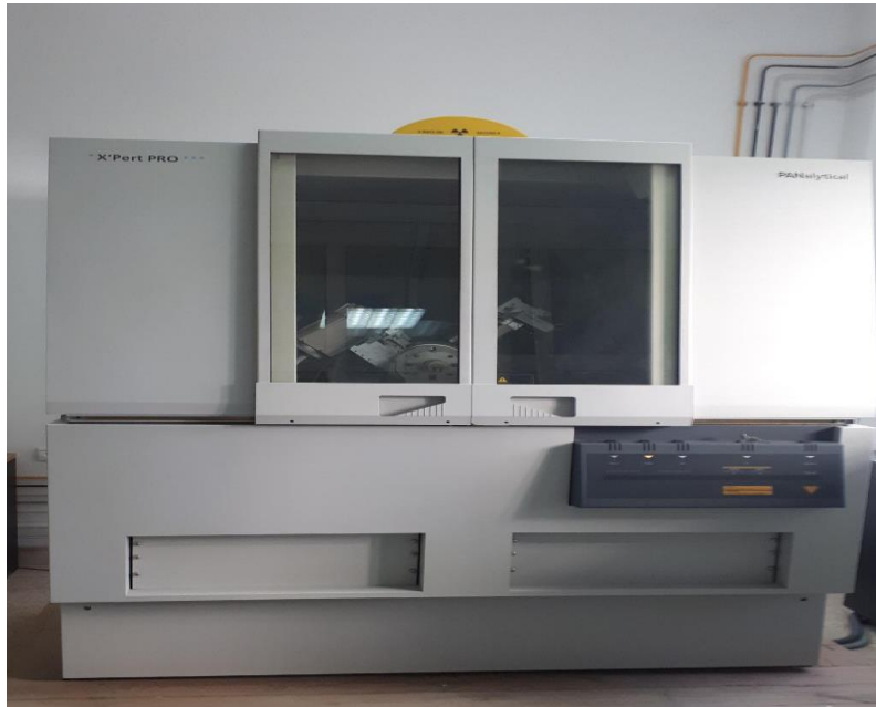
Figure II- 7 : Appareil d'analyse de diffraction des rayons X (X'Pert PRO Diffractometer on panalatycaI powder)
