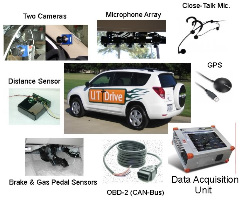
FIGURE 2.8: An instrumented vehicle used to collect naturalistic driving data (UTDrive corpus). Image downloaded from https://www.utdallas.edu/research/utdrive/corpus.html
