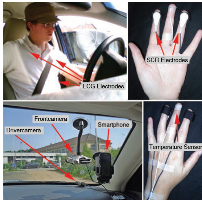
FIGURE 5.5: Sensors used for data collection in hcilab driving dataset
