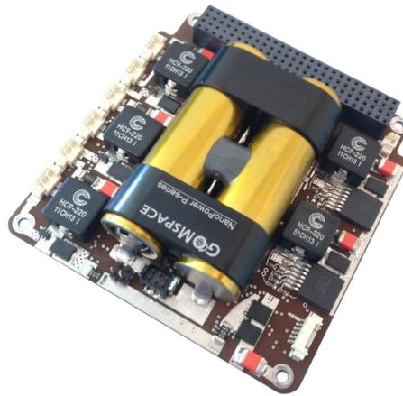
**Figure 3-18:** Module EdB GOMSpace Nanopower P31U [79]
