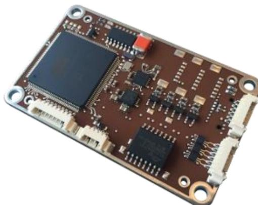
**Figure 4-15 :** Module GOMSpace NanoCom AX100 [89]
